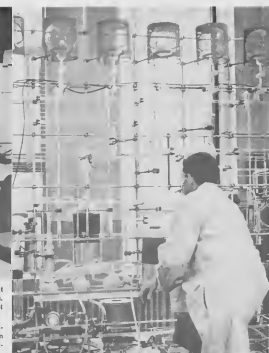
IMPROVED INSTRUMENTATION such as the mass spectrometer, above, is a constant tool of research men. The apparatus at right is used to conduct new tests on catalysts. Basic purpose of the device is to study the distribution of active sites on catalysts so that high octane gasoline can be refined as effectively as possible.
